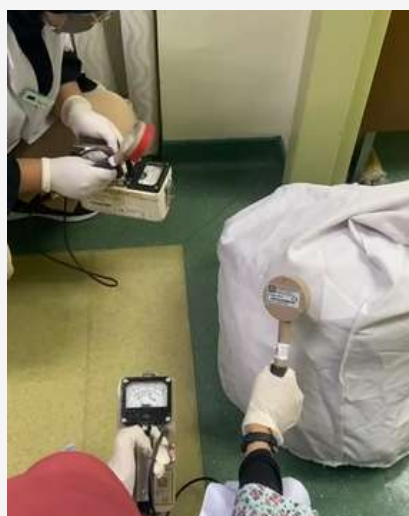
Figure 2: Radioactive waste measurement
