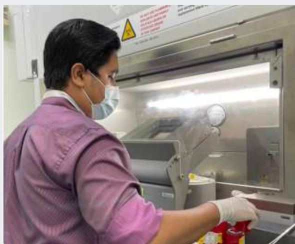
Physicist is demonstrating on how to place the radioactive source in the dose calibrator
