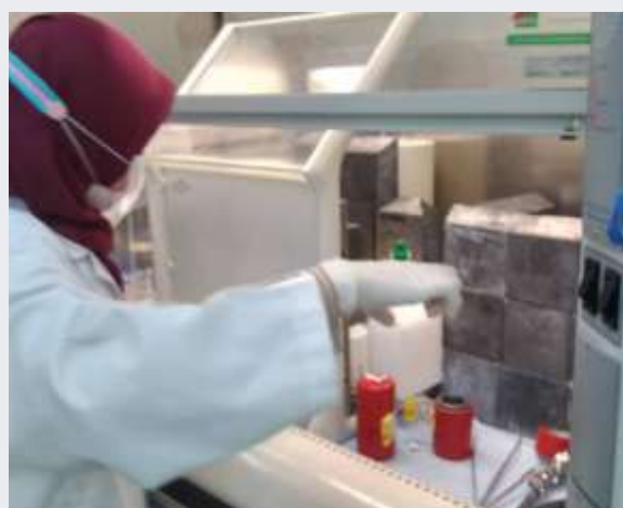
One of USM Trainee is placing the radioactive source using tweezers into the dose calibrator cylinder
