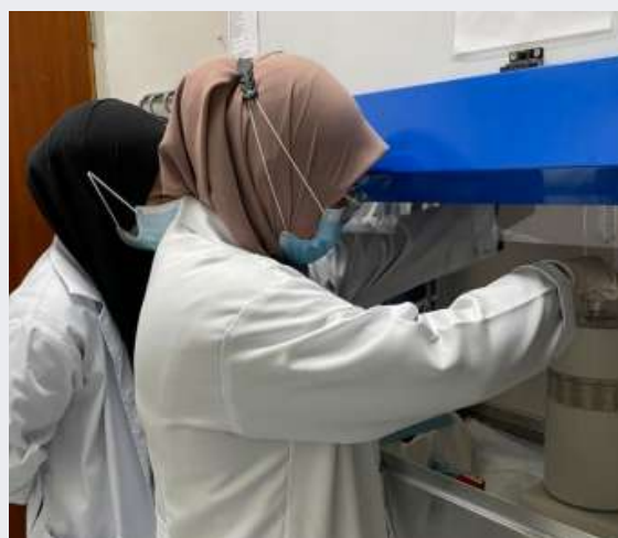
One of USM Trainee is placing the radioactive source using tweezers into the dose calibrator cylinder
