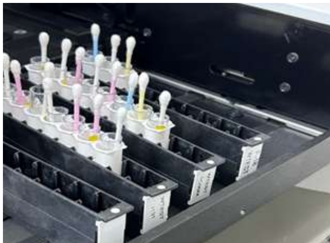
Figure 4: The samples placed in MCA to analyze for any contamination.
