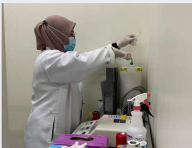
Physicist is demonstrating on how to place the radioactive source in the dose calibrator
